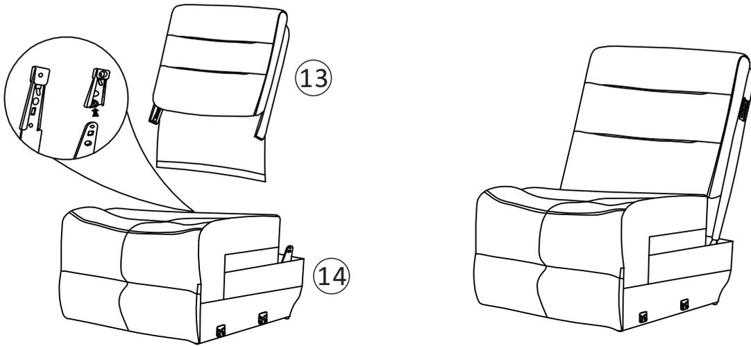
STEP 7: Install back ⑮ onto seat ⑰.
