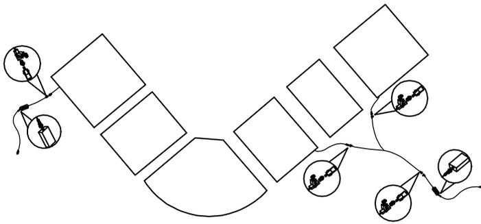
Safety Note: Transformer and cables are not to be placed under or within the recliner structure.
