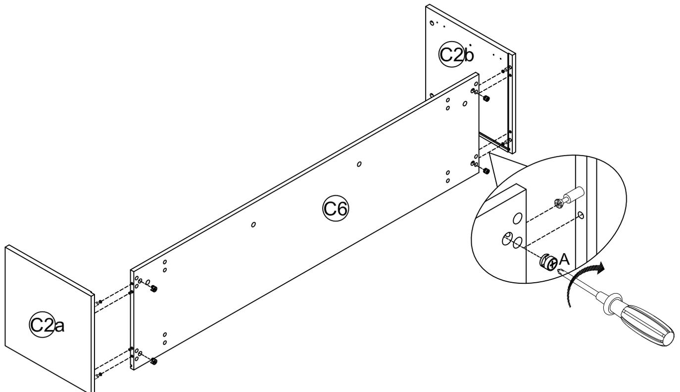
STEP 3: Insert the Dowel(B) to the Support Panel(C3),then assemble the Support Panel(C3) to the Bottom Panel(C6), Use a Phillips Head Screwdriver to turn the Cam Lock(A) to lock onto the head of Cam Pin(A),then Place the Cover(K) on the head of Cam Lock(A).
