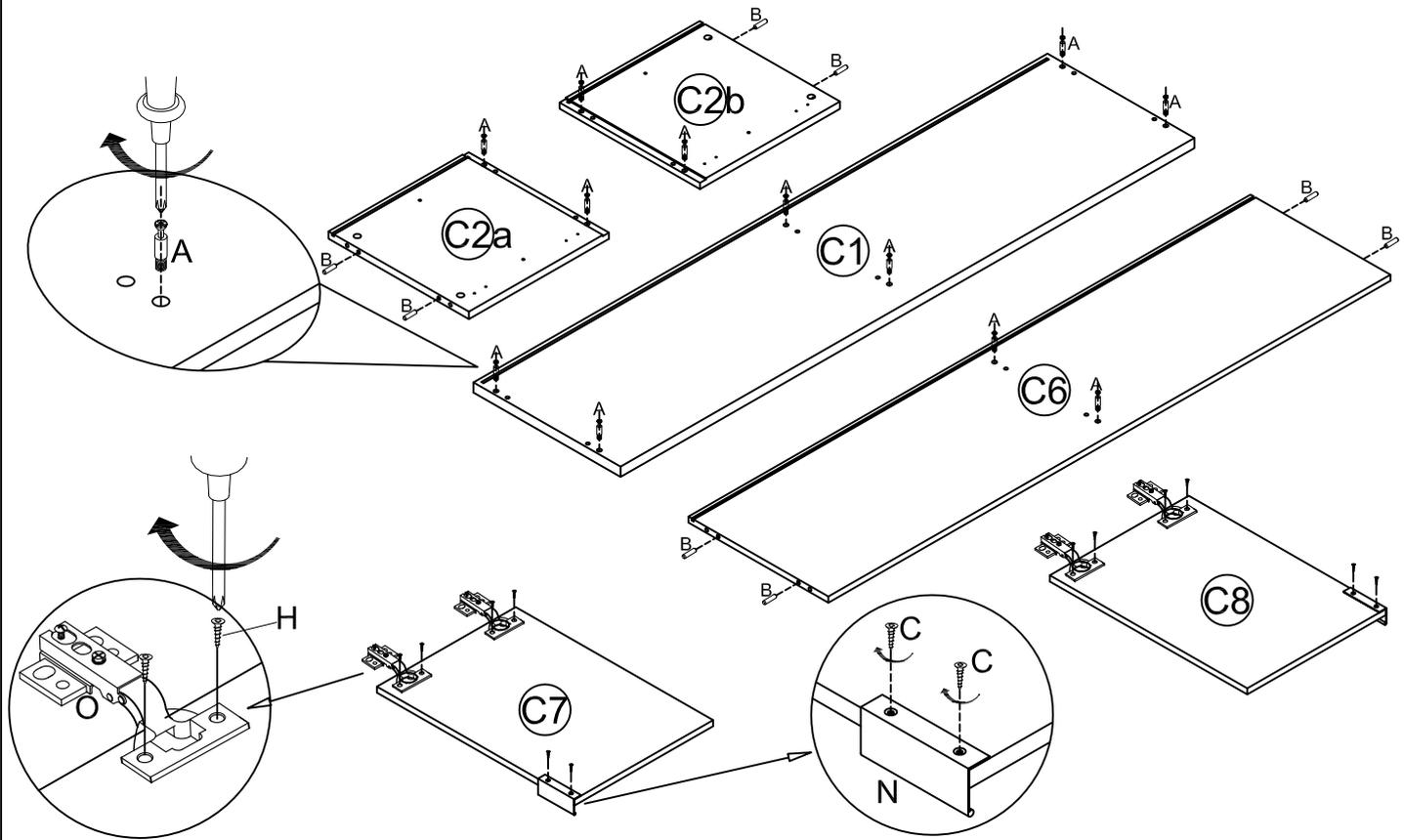
**STEP 2:** Assemble the Side Panel(C2a ,C2b) to the Bottom Panel(C6) ,Use a Phillips Head Screwdriver to turn the Cam Lock(A)to lock onto the head of Cam Pin(A).
