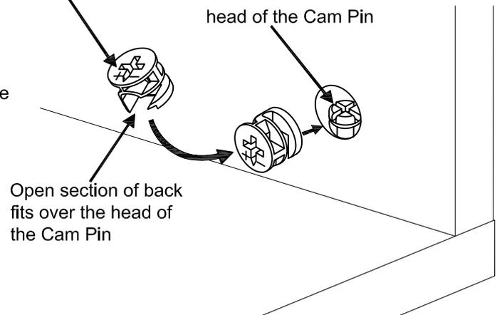
Open section of back fits over the head of the Cam Pin
