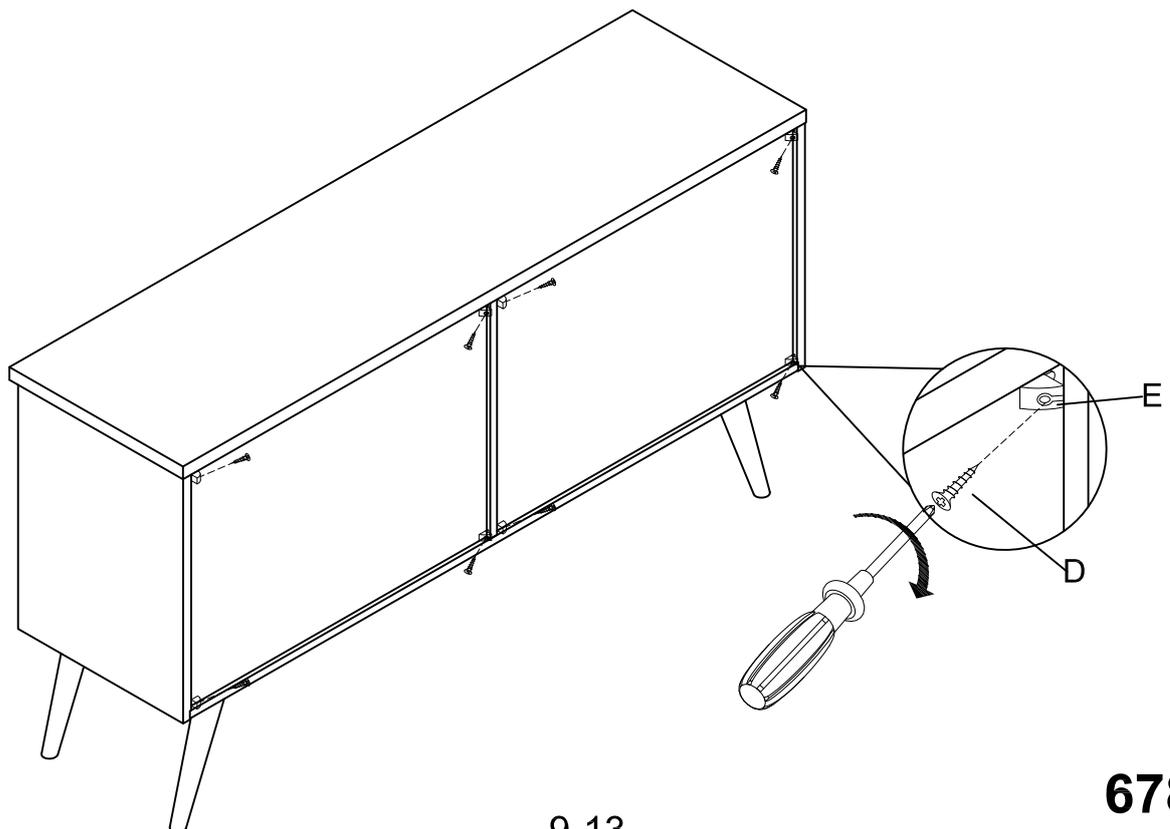
STEP 9: Use a Phillips Head Screwdriver to tighten the Hinge(O) to the Side Panel(C2a ,C2b) with Bolt(H).
