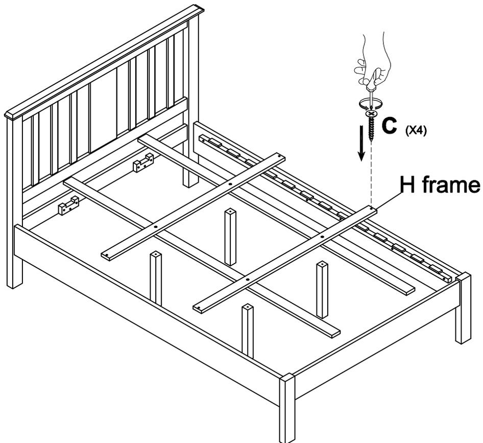
STEP 4: Attach **7** onto **3** using the screws (**C**), tighten it up by using a screwdriver.
