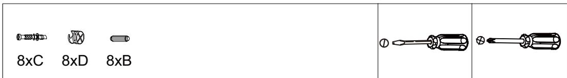
STEP 8: Fix top panel (7) to the body with dowel(B) and cam lock parts (C)&(D).
