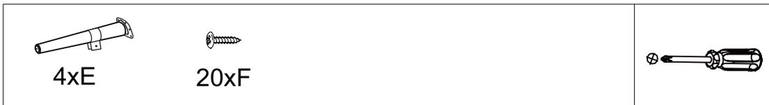
STEP 6: Install metal leg (E) to the body with screw(F).
