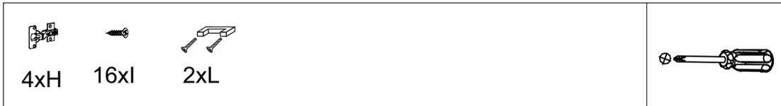
STEP 9: Install hinges and handle as shown in diagram.
