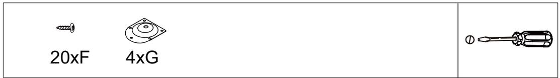
STEP 3: Fix metal plates(G) to panel(2) with screws(F).
