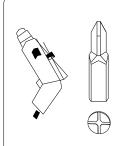
We recommend using a screwdriver to put this item together. However if you choose to use a power drill it must be used on LOW SPEED (LOW TORQUE) as too much pressure could damage the product
