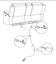
Safety Note: Transformer and cables are not to be placed under or within the recliner structure.
