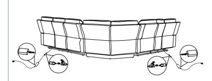
Safety Note: Transformer and cables are not to be placed under or within the recliner structure.
