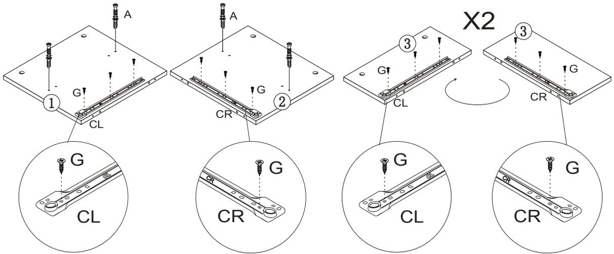
**STEP 2: Fix cam pin (A) to panel (5).
