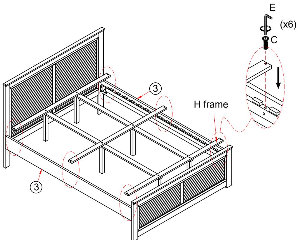
STEP 5: Once the bed is positioned and the support legs are adjusted to touch floor, the slats can then be laid down and secured before putting on the mattress.
