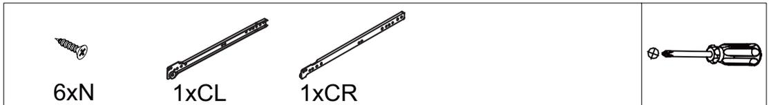
STEP 1: Install runner (CL)&(CR) to panel (2)&(3) with screws (N) .
