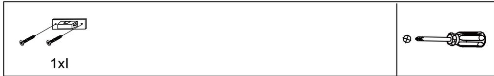
**STEP 1: Fix bracket to back panel using screws M3.5\*14MM .
