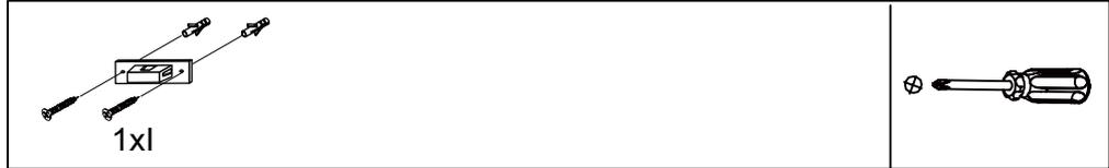
STEP 2: Fix bracket onto the wall using screws M4\*30MM.
