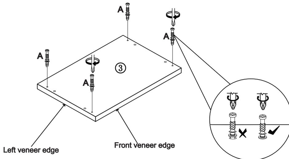
STEP 3: Attach top panel ③ to left side panel ① and right side panel ② with the cam locks ④ .
