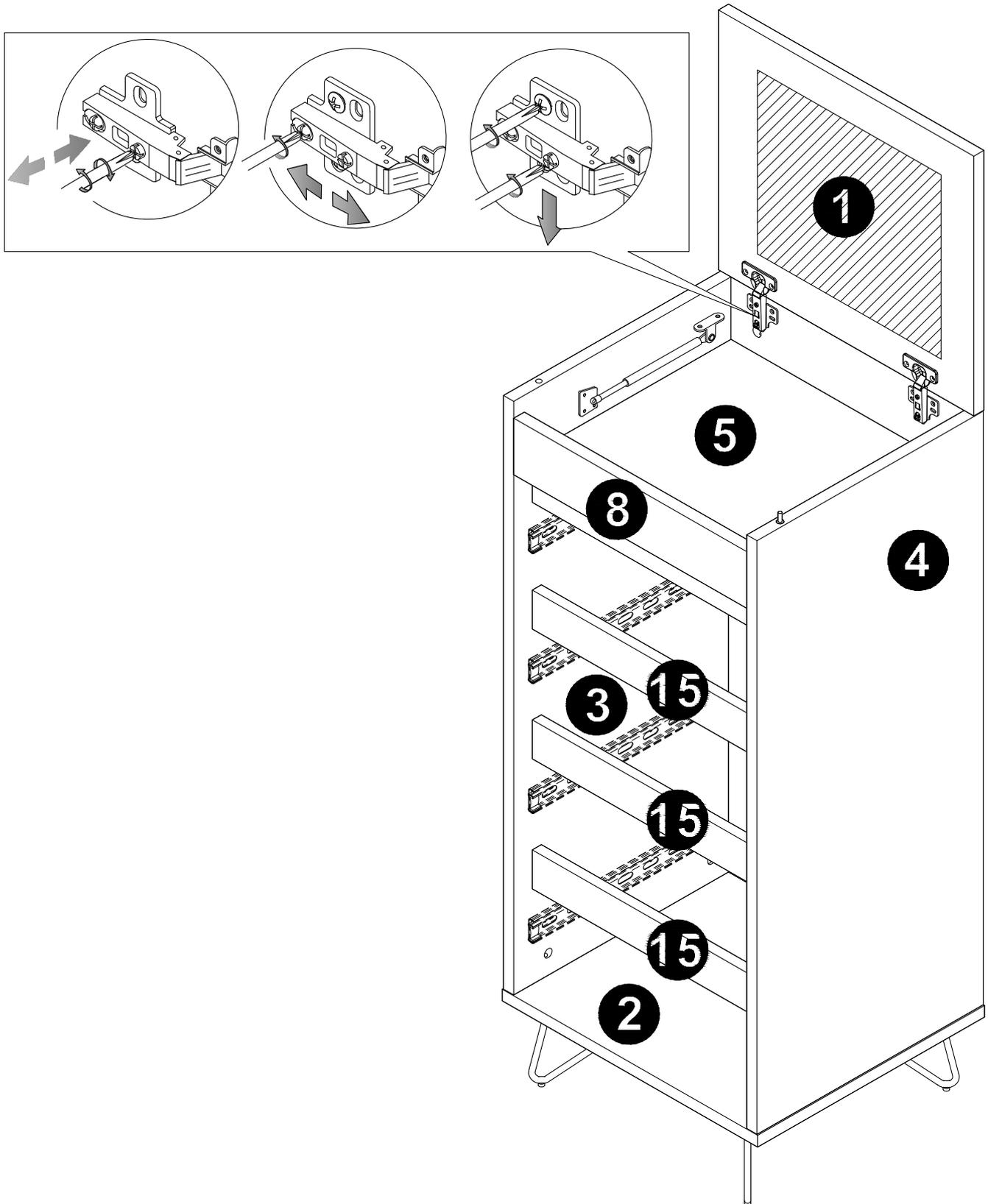
STEP 12: Attach pneumatic rod (S-2) to panel (1) with screw.
