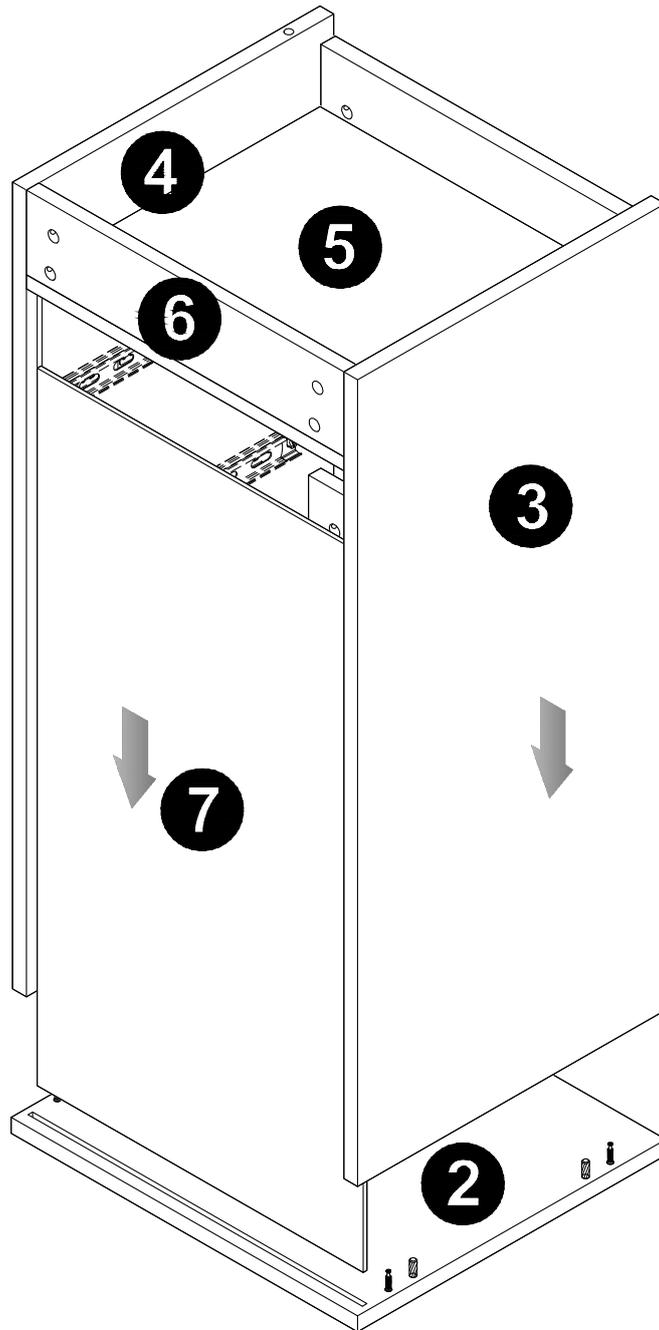
STEP 6: Fix panel (2) to panel (3) (4) with cam lock (C) .
