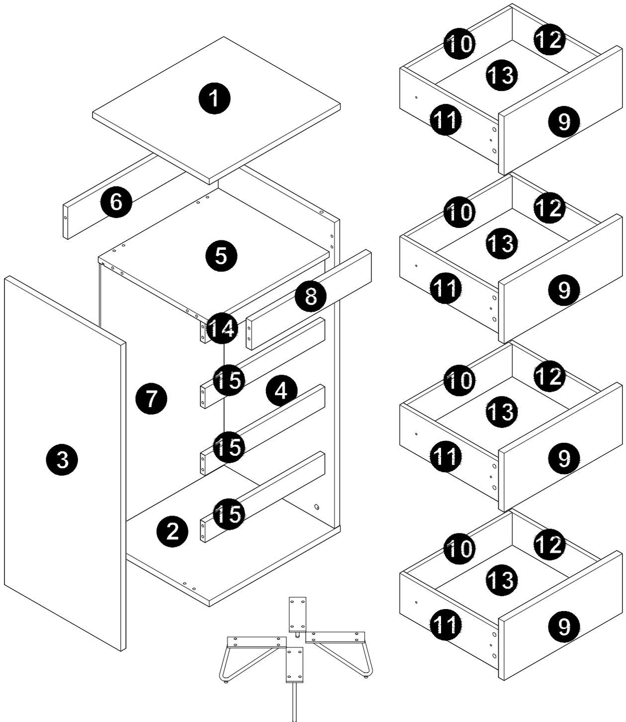
STEP 1: Fix dowel (B) and cam pin (A) to panel (2) (3) (4) (5).
