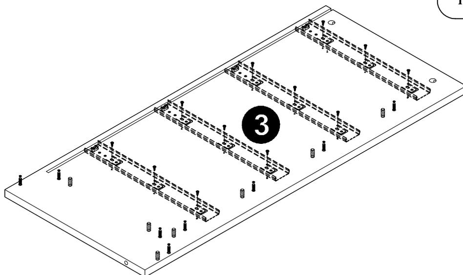
STEP 3: Fix panel (6) to panel (5) with cam lock (C).
