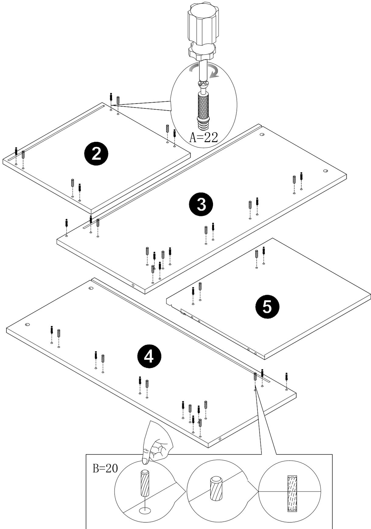
STEP 2: Fix rails (N-1) to panel (3) (4) with screw (V1) .
