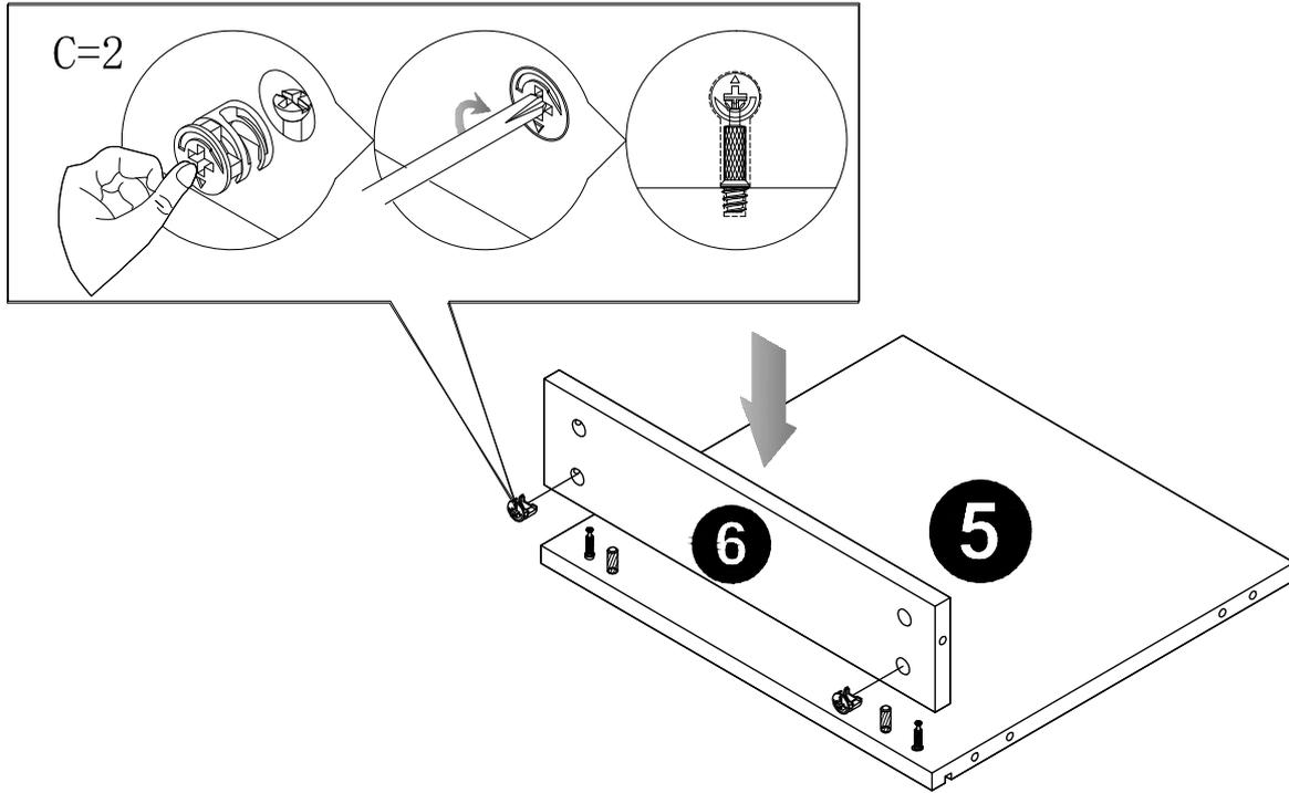
STEP 4: Fix panel (8) to panel (5) with cam lock (C) .
