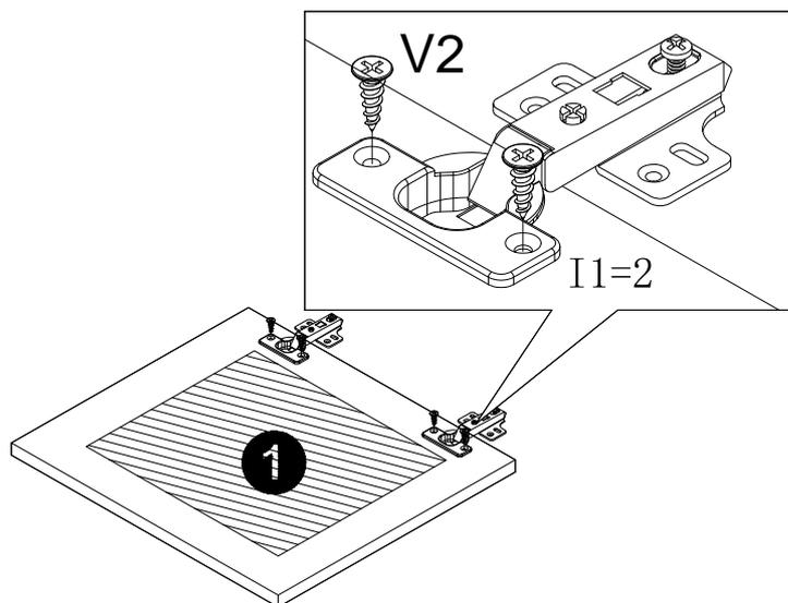
STEP 10: Fix top panel (1) to panel (6) with screw (V2).
