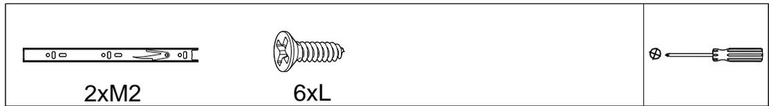
STEP 13: Fix runner(M2) to the drawer using screws(L).
