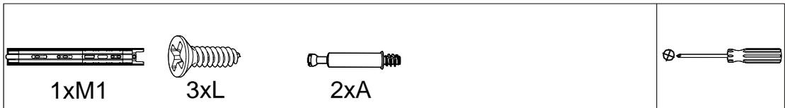
STEP 2: Fix runner(M1) to left side panel ② using screws(L). Fix cam bolts (A) to left side panel ②
