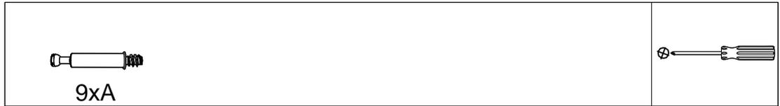
STEP 1: Fix cam bolts (A) to top panel ①.
