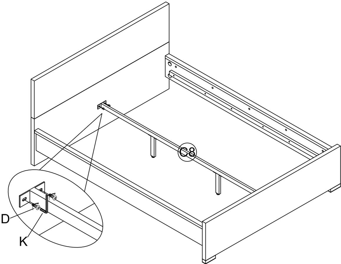
STEP 6: Use a Phillips Head Screwdriver to tighten the Slat (C7) to the Side Rail (C4) with Screw(F).
