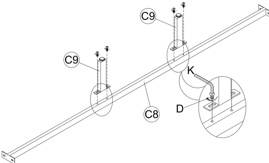
STEP 5: Use Hex Key (K) to tighten Centre Rail (C8) to the Headboard Bottom Panel (C2) and Footboard Panel (C3) with Bolt (D).
