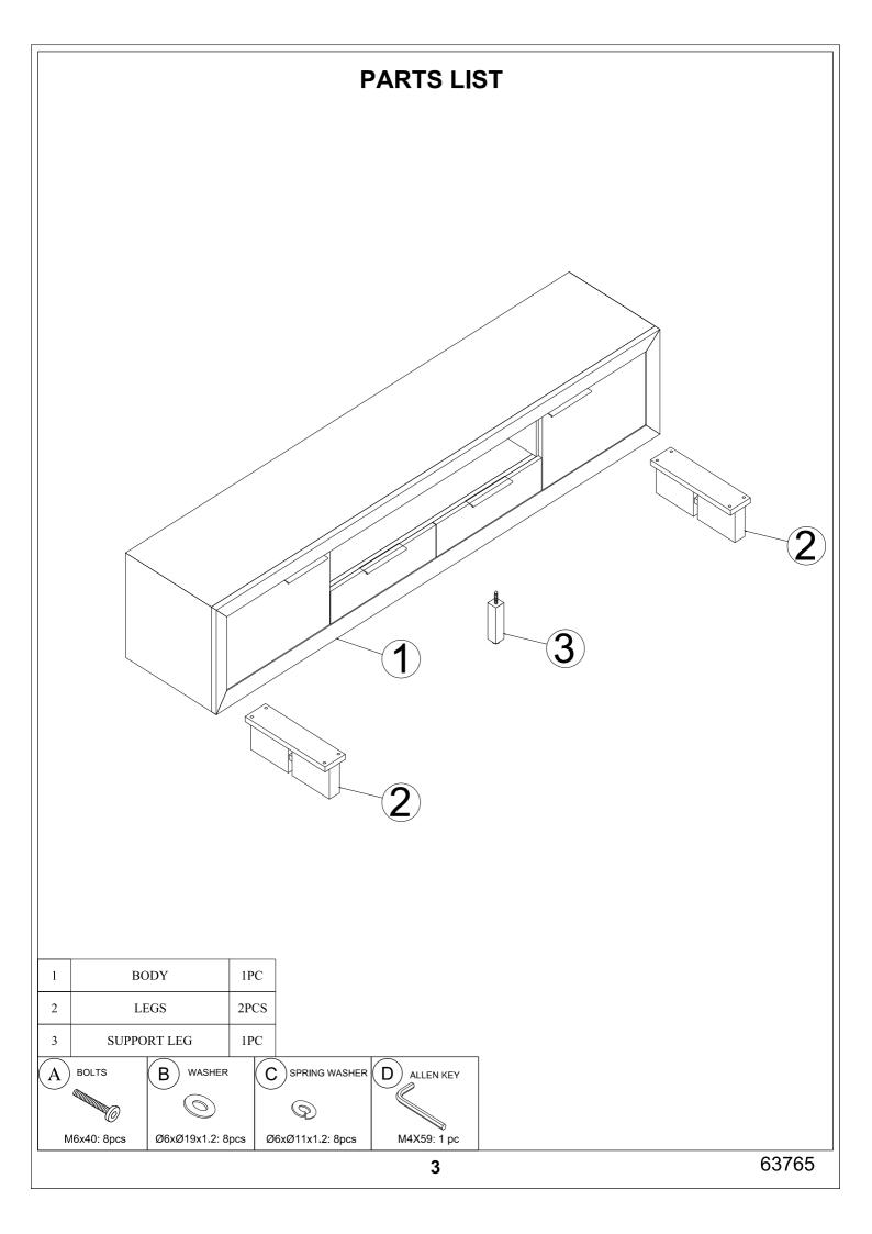
Step 1: Fasten the legs (2) To the body (1) with bolts (A), washer (B), spring washer (C) and using allen key (D)
