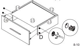
2:Join side panels (13)(14) and back panel(12) with screws (A).
