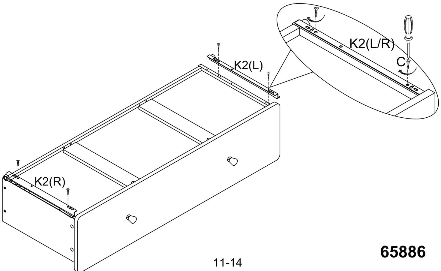
STEP 13: Insert the Drawer to the Left Side Panel (C2a) and Right Side Panel (C2b).
