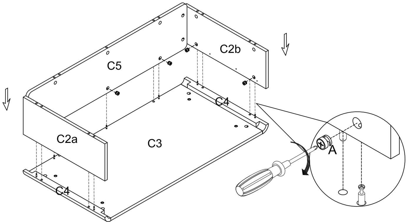
STEP 6: Use a Phillips Head Screw driver to assemble the Runner (K1L) to the Left Side Panel (C2a) and assemble the Runner (K1R) to the Right Side Panel (C2b) with Screw )C). Assemble the Back Panel (C5) and the Left Side Panel (C2a) and Right Side Panel (C2b) to the Top Panel (C1) and Corner Panel (C4). Use a Phillips Head Screw driver to turn the Cam Pin (A) the Cam Lock (A).
