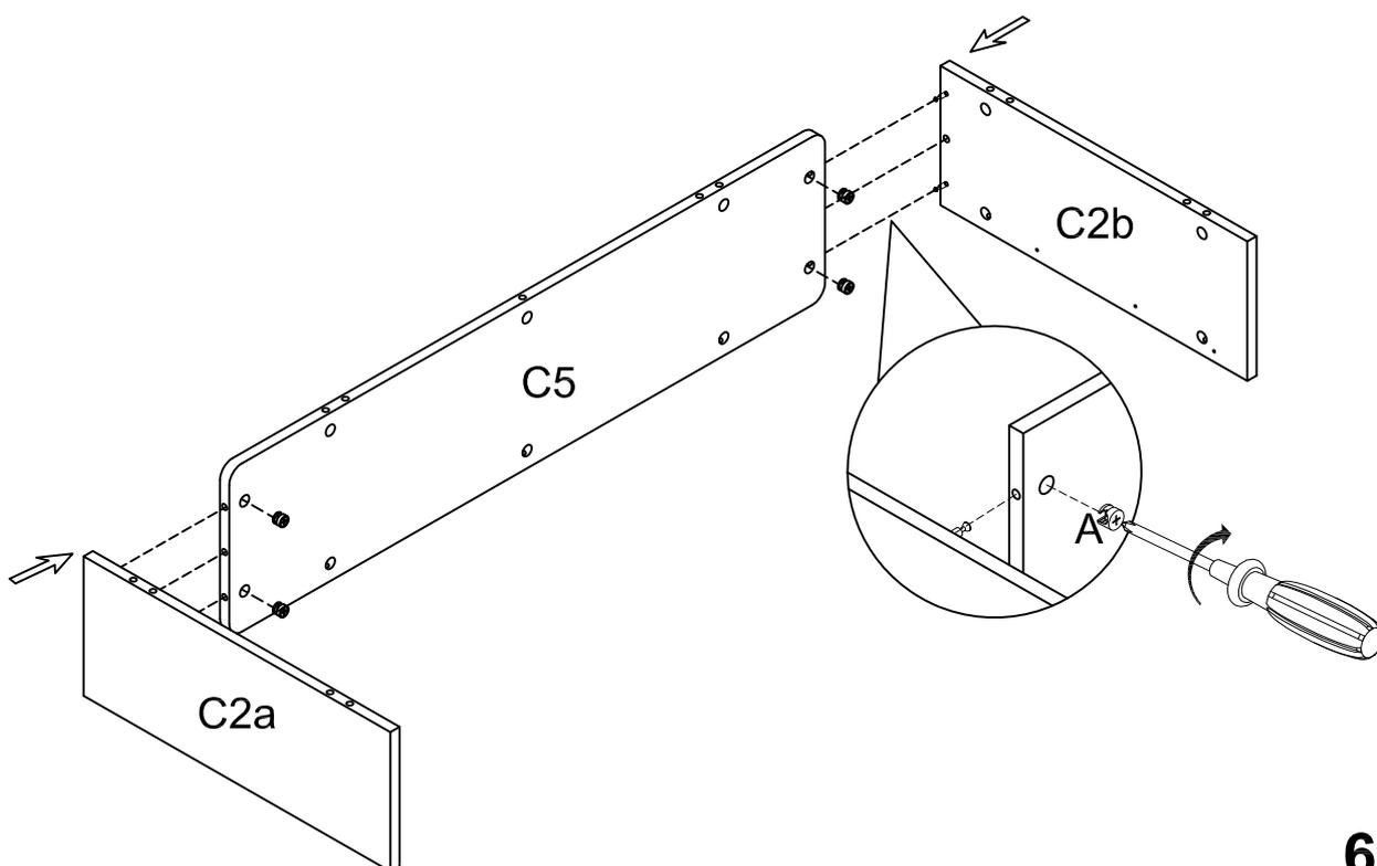
STEP 5: Assemble the Back Panel (C5) and the Left Side Panel (C2a) and Right Side Panel (C2b) to the Bottom Panel (C3) and Corner Panel (C4). Use a Phillips Head Screw driver to turn the Cam Pin (A) the Cam Lock (A).
