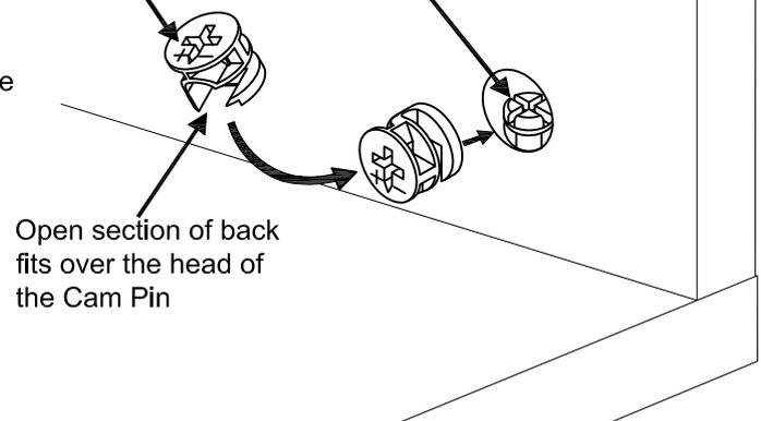
Open section of back fits over the head of the Cam Pin
