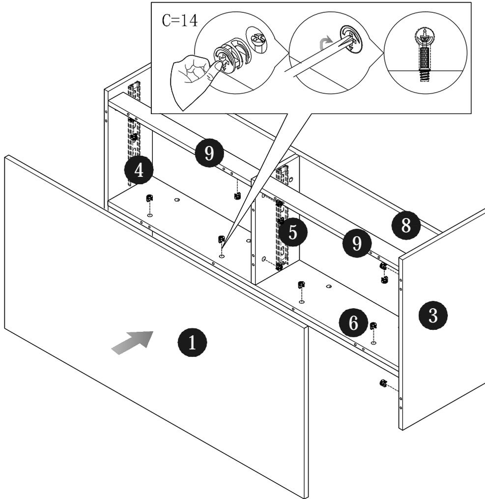
STEP 6: Fix panel (2) to panel (3) (4) (7) with screw (Q).
