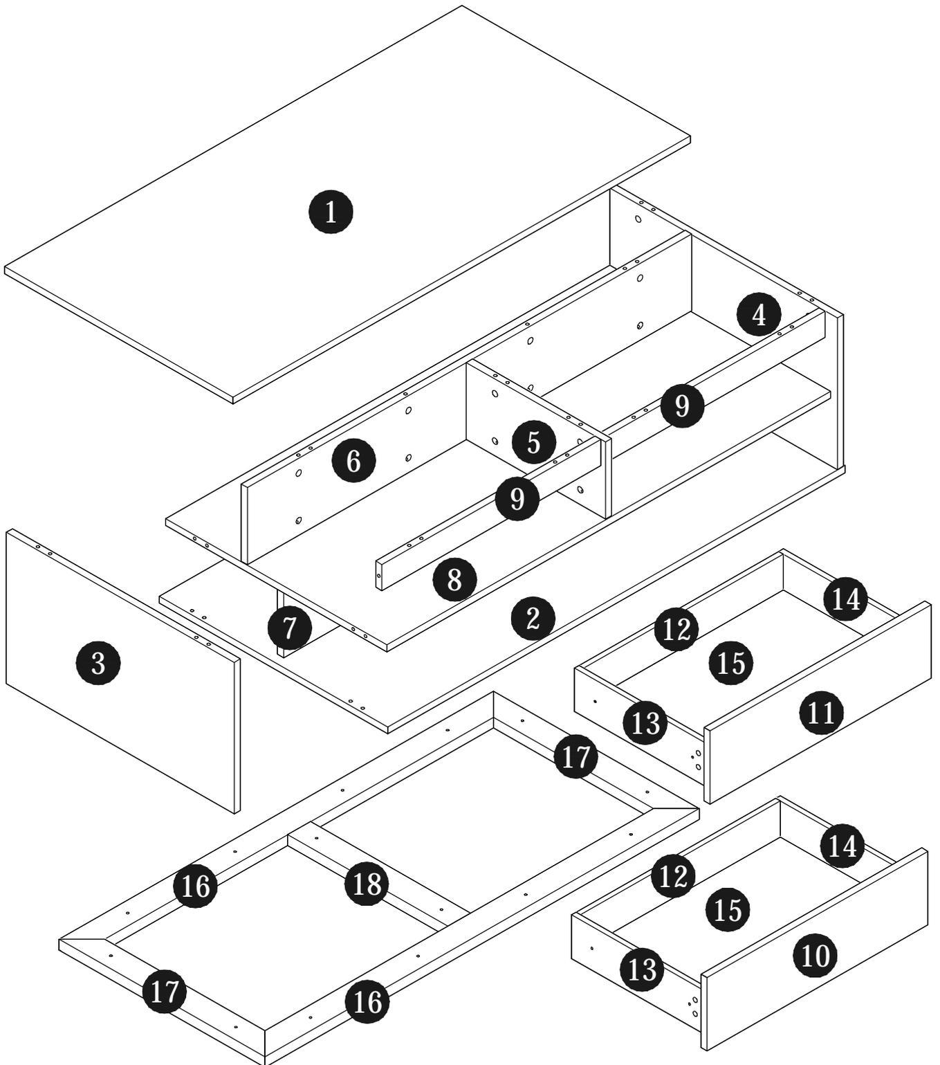
STEP 1: Fix rails (N-1) to panel (3) (4) (5) with screw (V1) .
