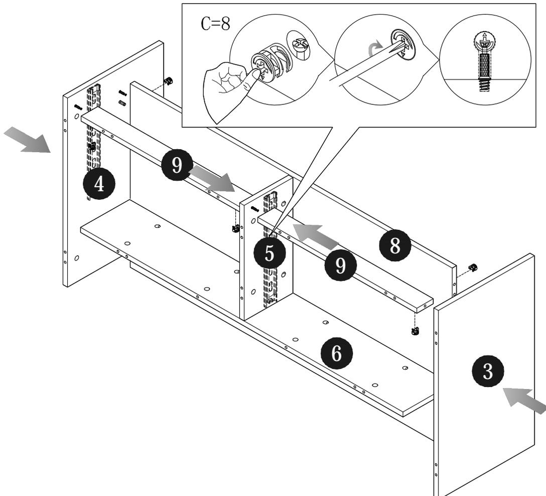
STEP 5: Fix panel (1) to panel (3) (4) (5) (6) (9) with cam lock (C).
