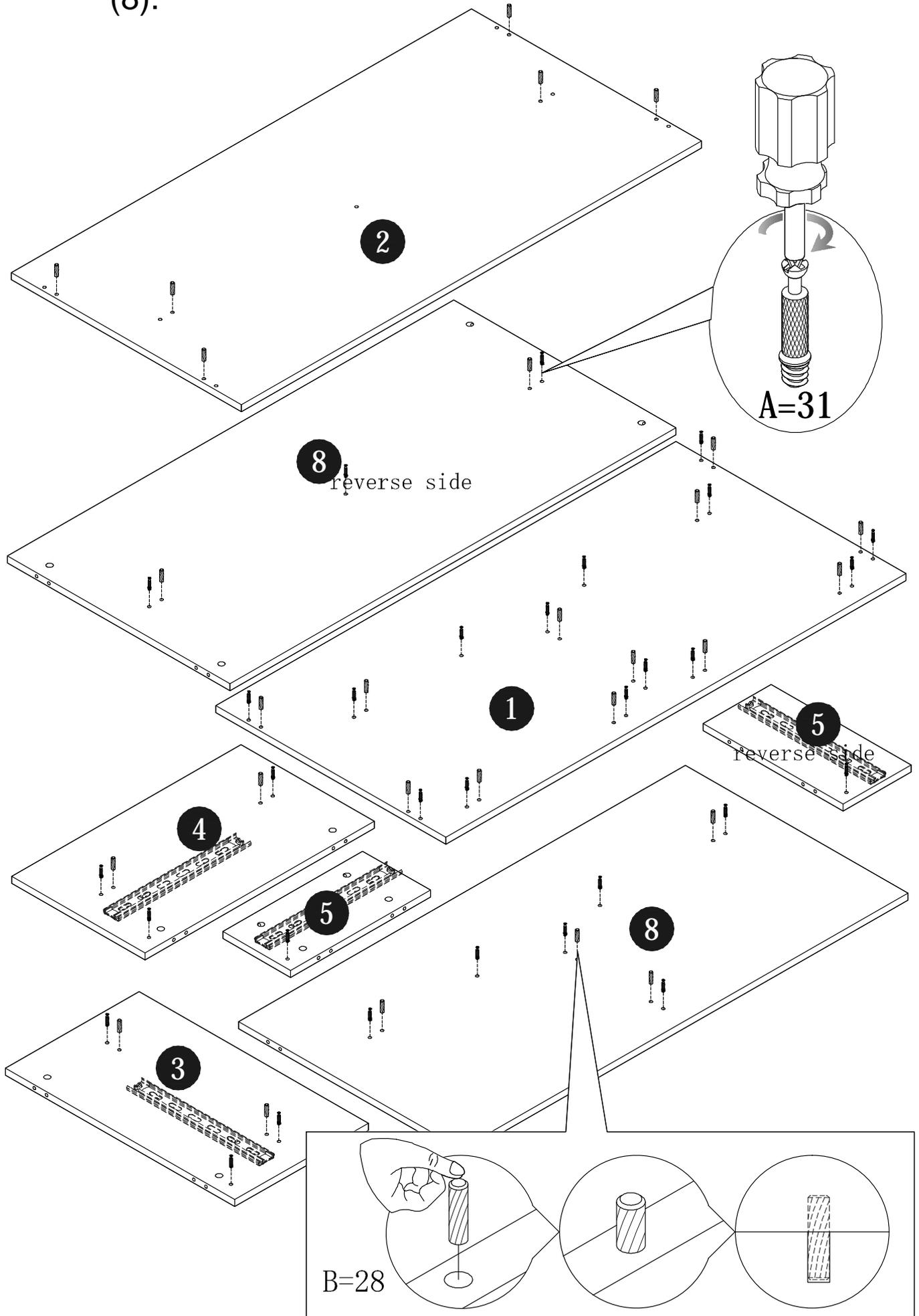
STEP 3: Fix panel (5) (6) (7) to panel (8) with cam lock (C).
