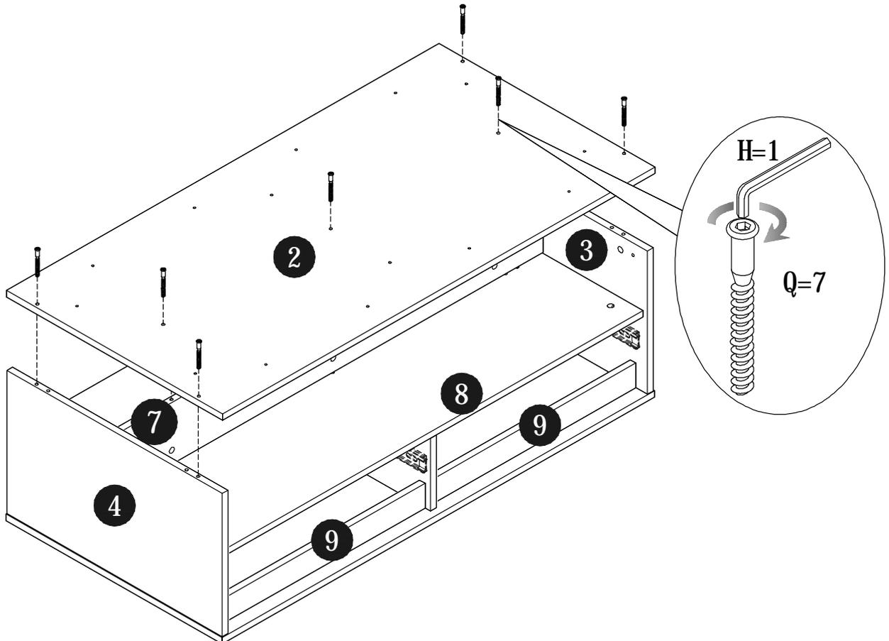
STEP 7: Fix panel (16) (17) (18) to panel (2) with screw (V3).
