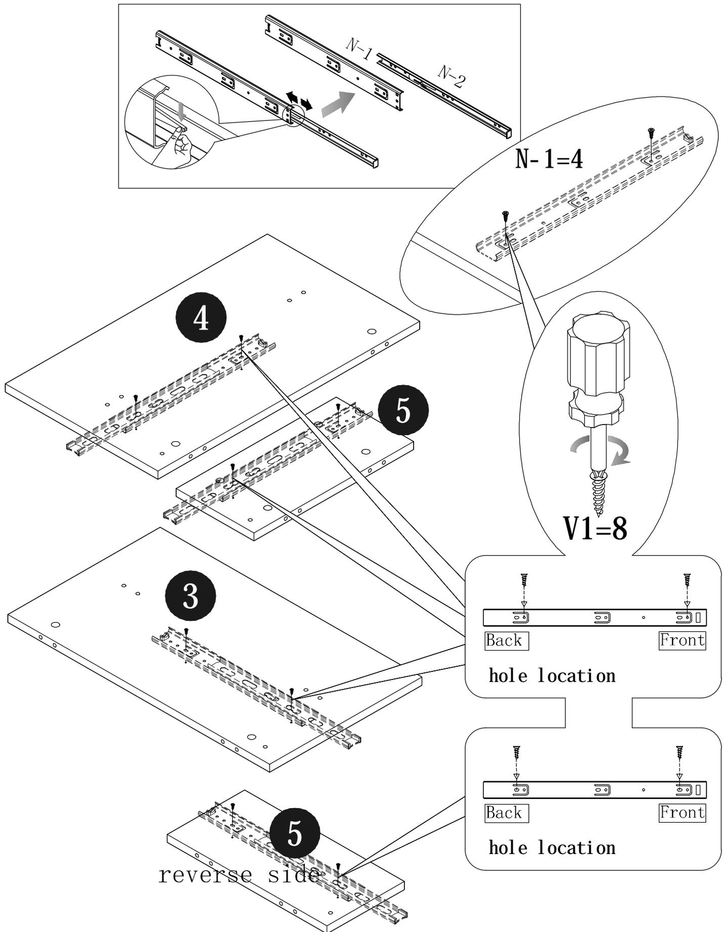
STEP 2: Fix dowel (B) and cam pin (A) to panel (1) (2) (3) (4) (5) (8).
