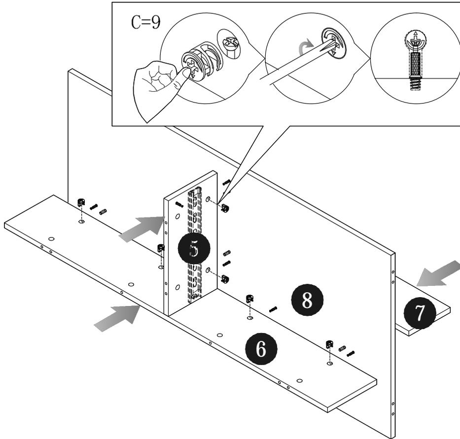
STEP 4: Fix panel (9) to panel (3) (4) (5) with cam lock (C).
