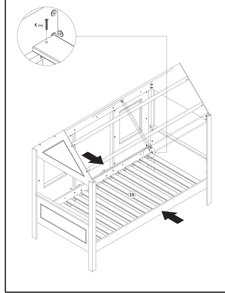
Attach and secure all **Roof Top Panel** onto previous assembly by following our suggested order starting from **1** and ending with **8** as indicated inside arrows by using **Screws (L)**, tighten it up by using a Crosshead Screw Driver. Go on to complete the entire assembly.
