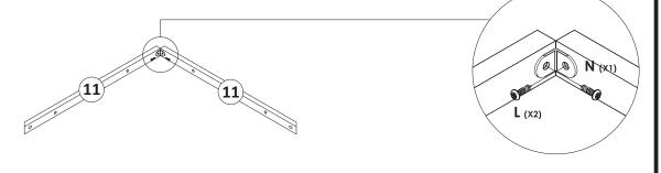
Align both the attached Roof Support Rail (Short) towards the center of assembly based on marking holes given.
